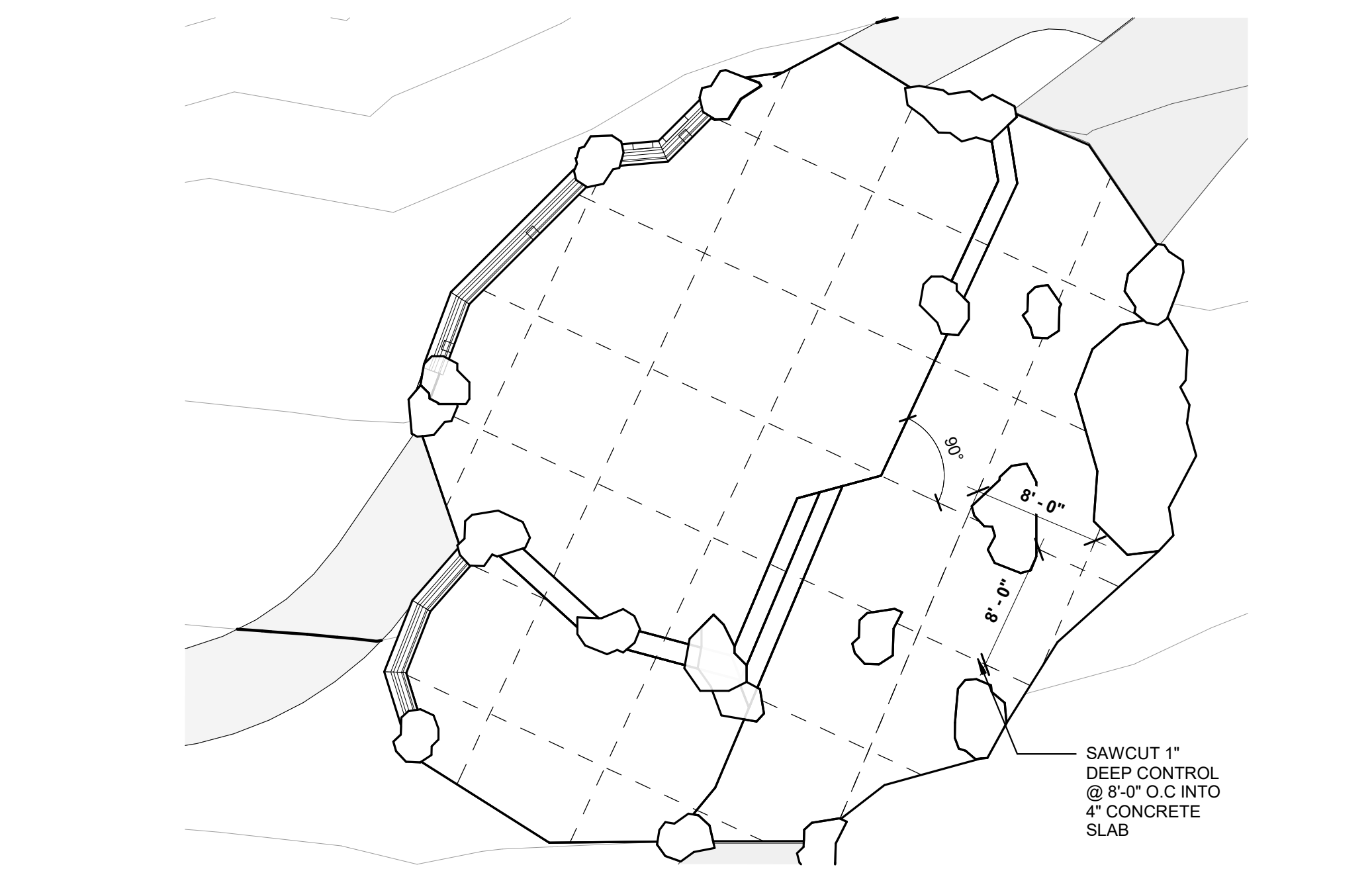
6 CONTROL JOINT DIAGRAM 1/8" = 1'-0"
